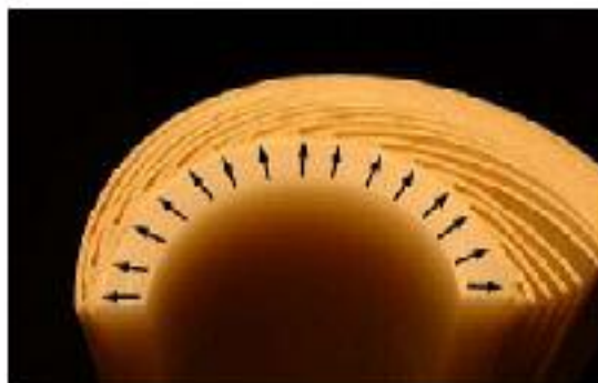
Figure 1.14 Cross-section of a permeate water tube through the side glue lines of the leaves (arrows indicate even spacing of leaves)
